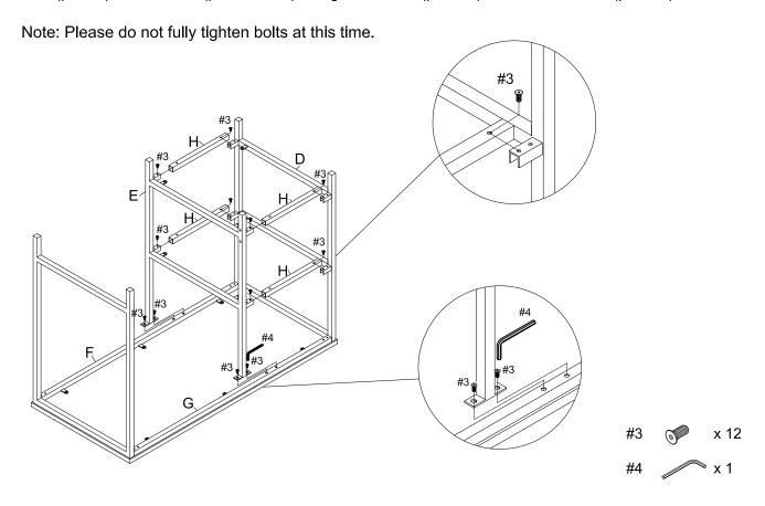
Step 3. Attach bottom rail (part I) between left panel (part C) and middle panel (part E) using sunk bolts (part #3) and allen wrench (part #4).
