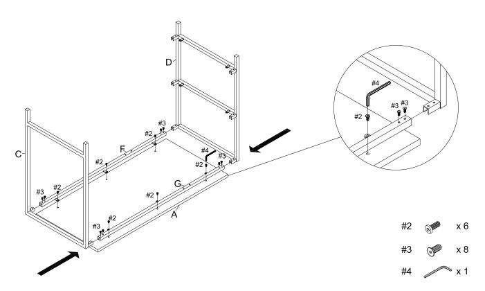
Step 2. Attach shelf rails (part H) into right panel (part D). Attach middle panel (part E) by inserting into shelf rails (part H) then to rails (parts F & G) using sunk bolts (part #3) and allen wrench (part #4).
